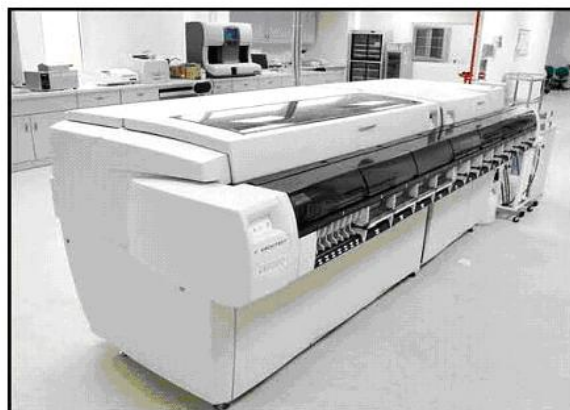
Figure 4 – Example of an Automated ELISA System
